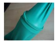
5. Position Sleeve O ring over Glovezon cone and pull tight.
