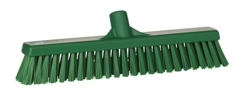
This sweeping broom has two types of bristles. When pushing the broom forward the front rows, which have firm bristles, loosen the dirt and push heavier debris. The softer bristles of the back rows, gather the finer particles. It is suitable for all areas in kitchens and restaurants.
