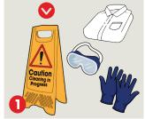
Place safety Sign & equip with the appropriate PPE as indicated in the SDS.
